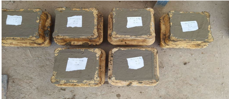
Figure 4 – Concrete made in 15x15x15 cm 3 cubic test specimens
