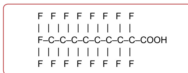
Figure 1: Simplified chemical structure of perfluorooctanoic acid (PFOA), showing a fully fluorinated carbon chain and a carboxylic acid head group
