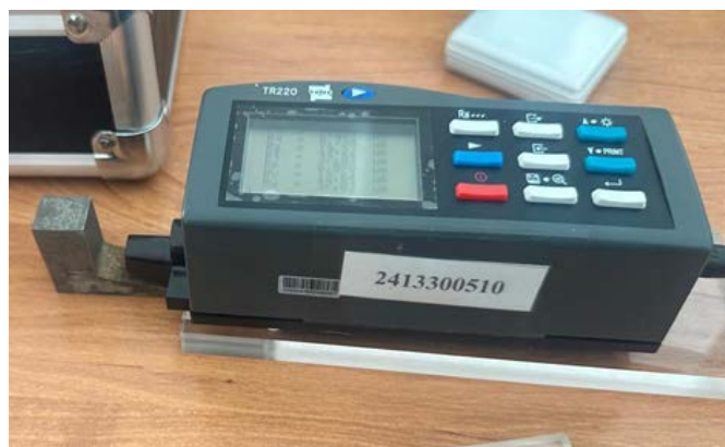
Fig. 6. Tooth sample roughness measurement process
