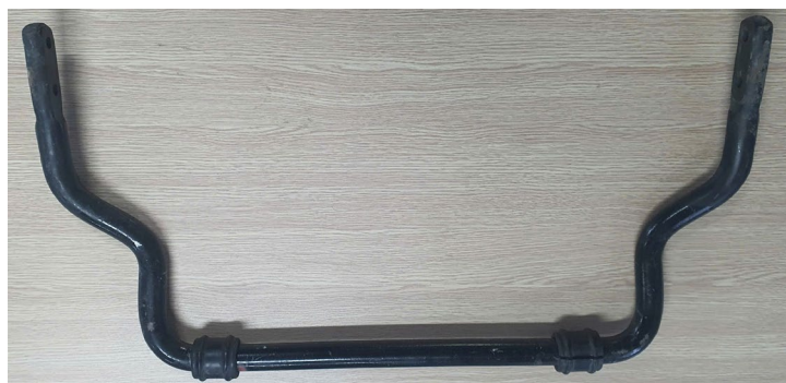
Fig. 2a. Shape of the anti-roll bar in trucks: a) actual manufactured bar, b) geometric diagram of the bar
