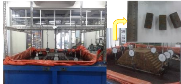
Figure 2: Laboratory small-scale model for embankment load test
